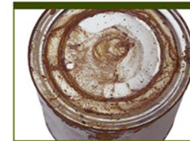
Rust that cannot be wiped off
